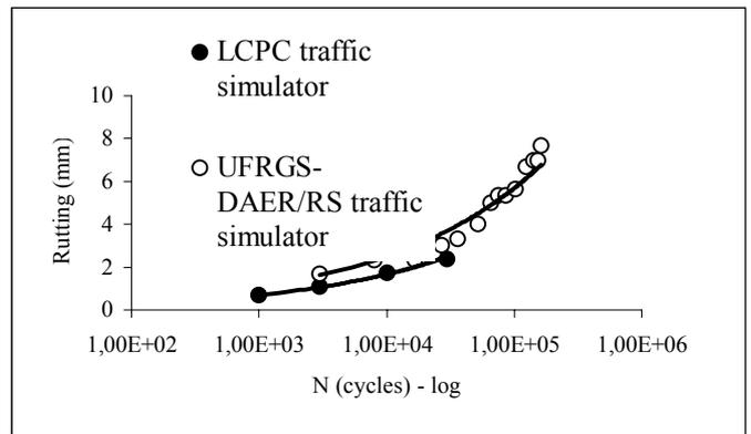
Figure 7. Comparison of rutting evolution using both traffic simulators
