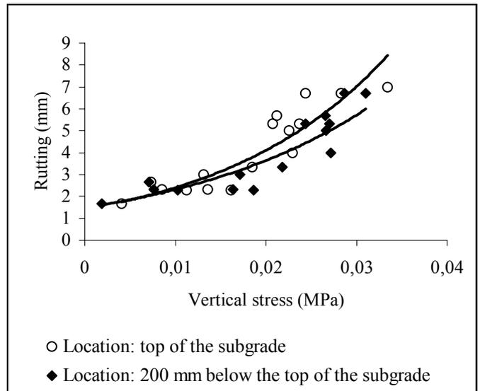
Figure 8. Rutting as a function of measured compressive stress
