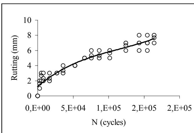
Figure 6. Rutting evolution in a test section loaded by UFRGS-DAER/RS traffic simulator
